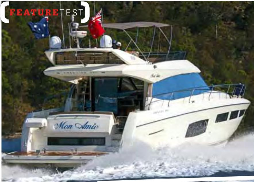
The hydraulically-lowered swimplatform (right) makes accessing the water almost too easy. Just press a button and launch the tender.
